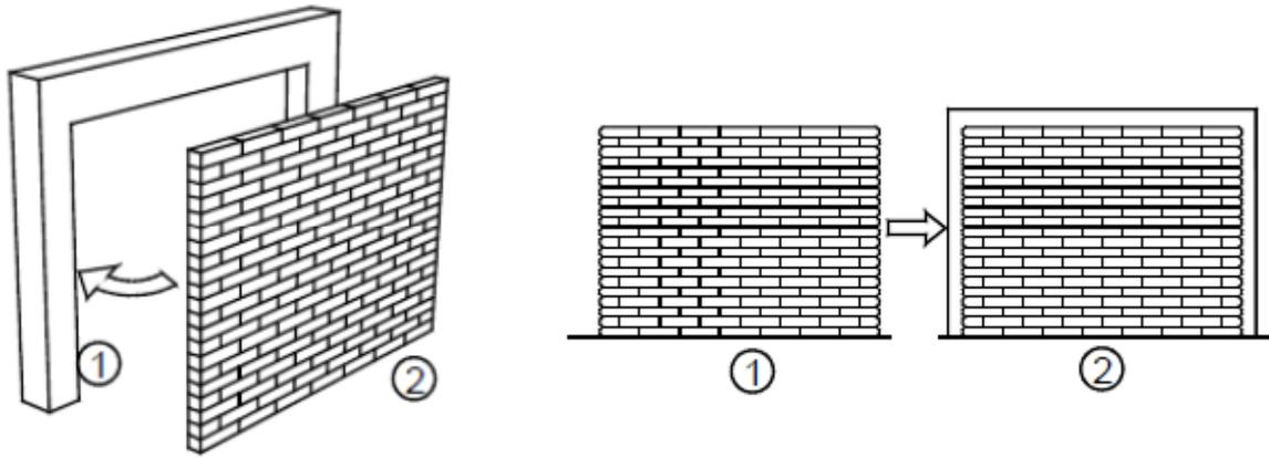
Construction sequence for infill (left) and confined masonry (right); Images courtesy Confined Masonry Network
